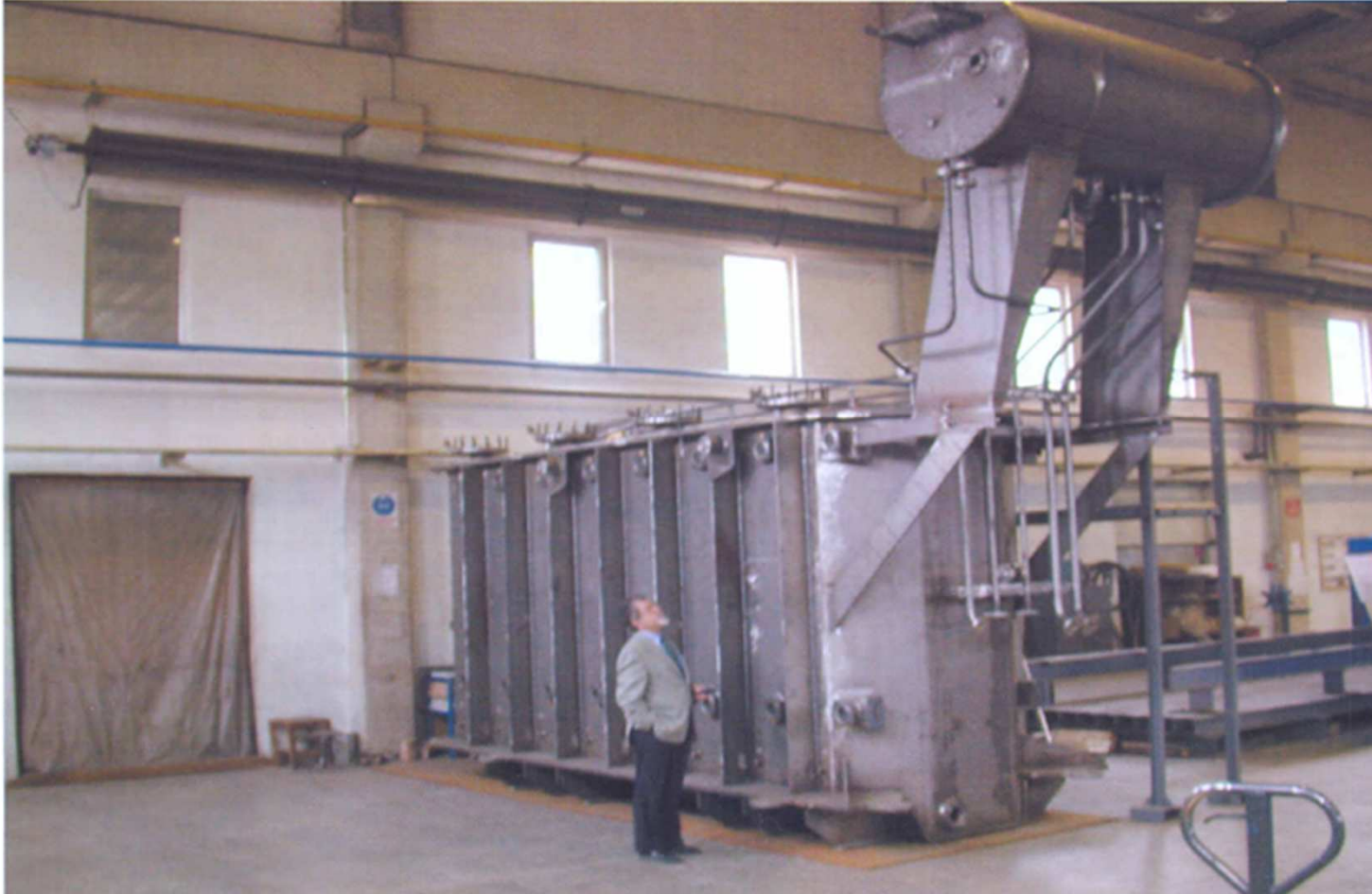
TANKS FOR HIGHVOLTAGE POWER TRANSFORMERS
