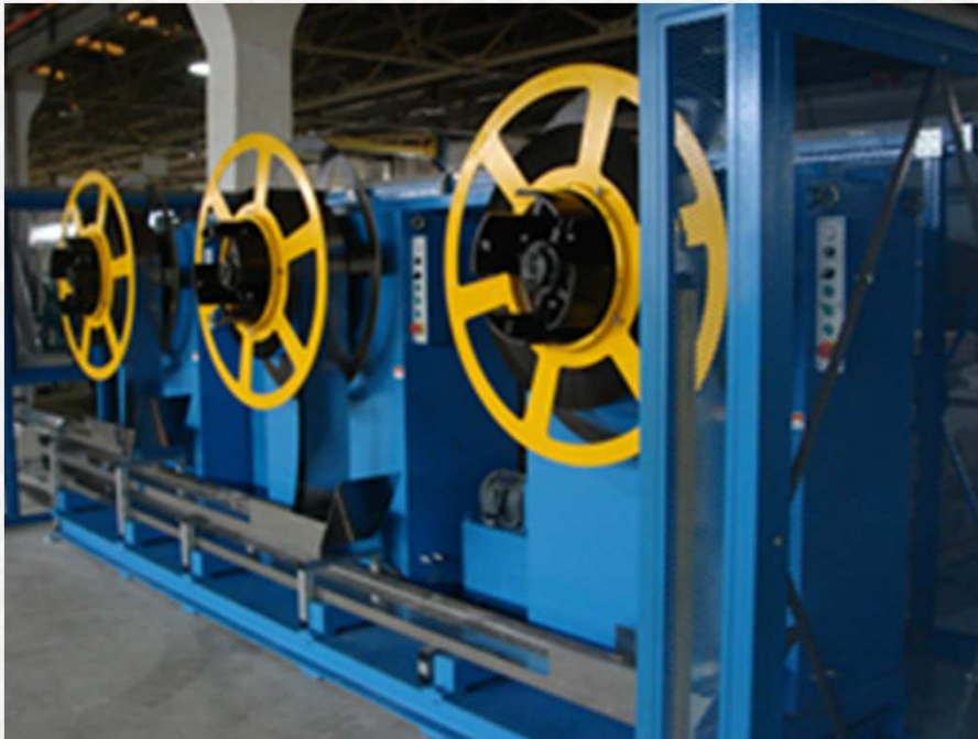
Progressive Cutting Line of the ribbon
