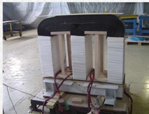
Measuring of the core losses
