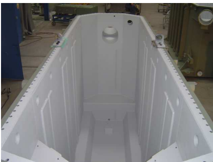
Assembling of the shunts on the tank wall
