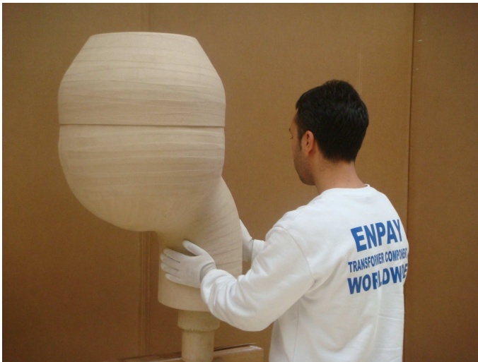
Position of 500 kV lead exit with barrier system in the Tank Connection to winding at the top
