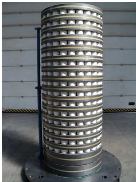
Core Limb for 1200 kV 300 MVAR shunt reactor
