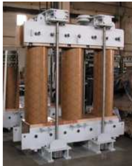
Fig. 8 - 3 Limb Reactor Core clamped on the side
