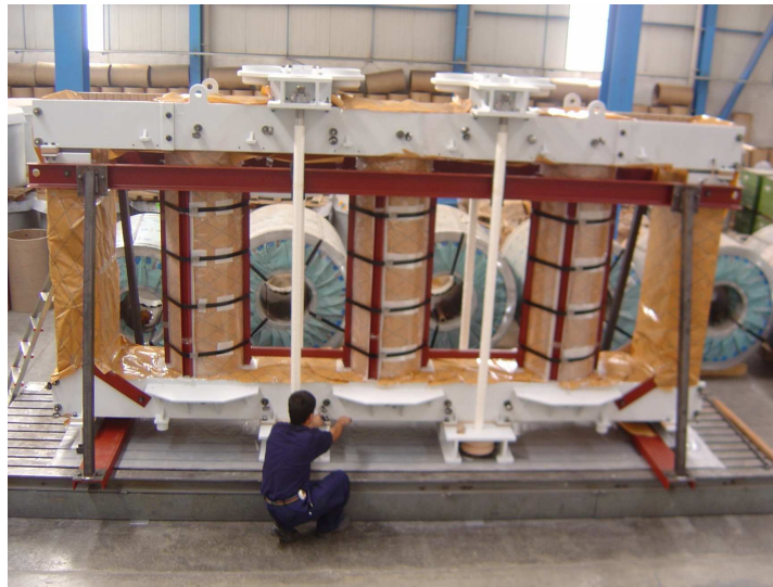
Fig. 7 - 5 Limb Reactor Core clamped on the side
