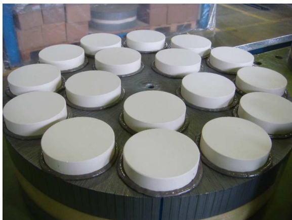
Fig. 2 Core Package for Longitudinal Rod clamped on the side
