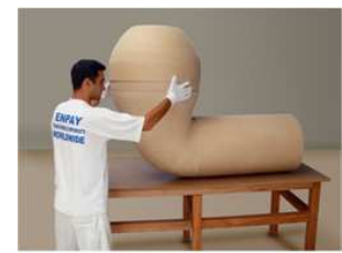
Fig.14. 1200 kV Lead Exit BIL: 2300 kV – SIL: 1675 kV (for inside of tank design )
