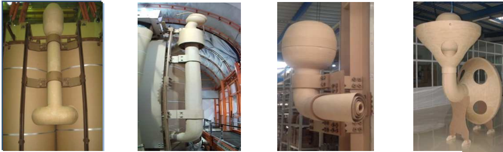
Figure4. Different type of lead exit designs for different voltages, from mid or upper of HV windings
