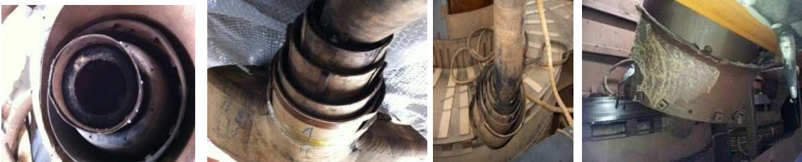
Figure9. Burned bellows and upper leads of HV winding
