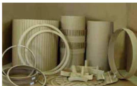
Figure1. Insulation parts of HV transformer
