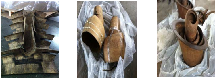
Figure10. Burned snouts, electrodes, bellows
