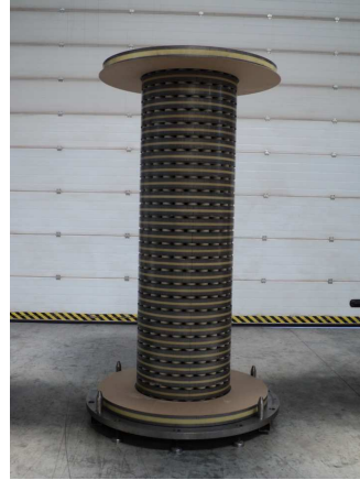
Bevel edge core limb and additional ring yokes of a single ph. reactor
