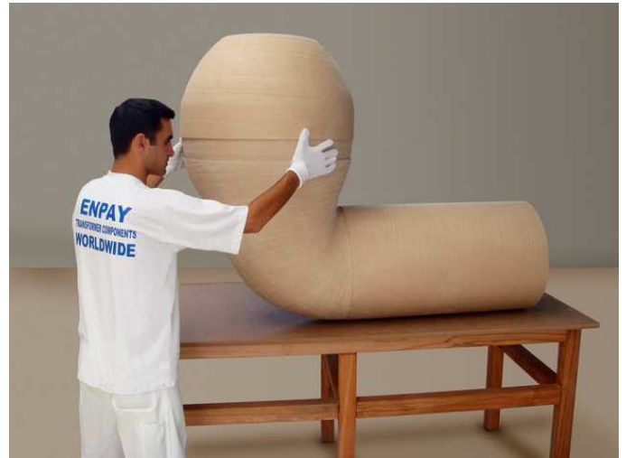
1200 kV Lead exit for test transformer
